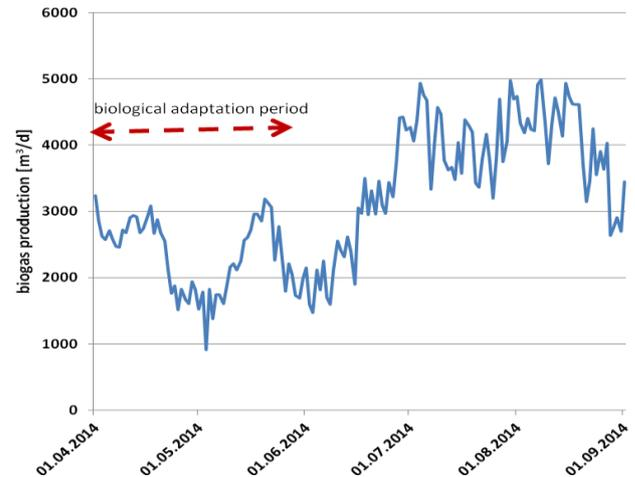
Figure 3: Demo Installation at Shek Wu Hui STW. A 5 kW ULTRAWAVES ultrasound reactor unit as plug&play system in a 10´-container is operating since April 2014. After the typical adaptation period we can observe an increase in biogas production.
