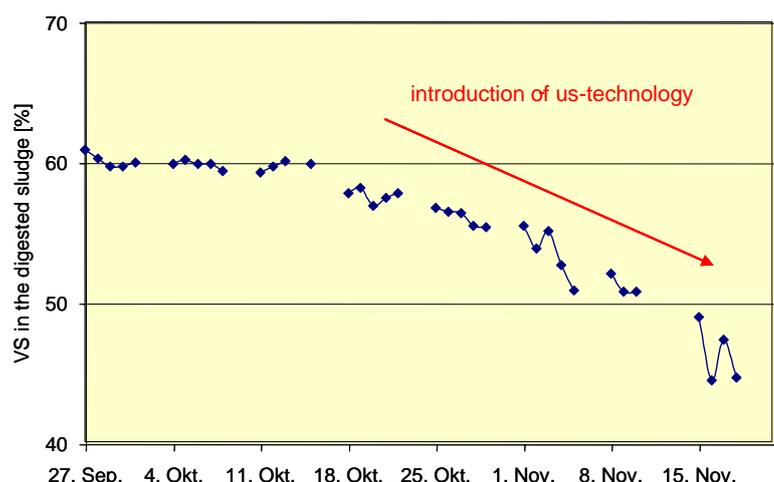
Figure 1: Installation at Meldorf WWTP and results. The volatile solids (VS) in the digested sludge were significantly reduced in conjunction with the introduction of ultrasound technology at Meldorf WWTP. Analyses reveal that the VS content of the digested sludge was reduced from 60% to 45% over the course of the test period.
