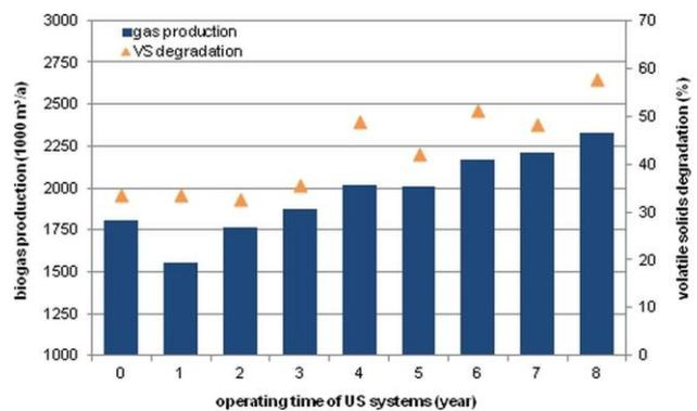
Figure 2: Installation at Bamberg WWTP and results. By using the ULTRAWAVES ultrasound systems the degradation of the organic sewage sludge components was increased from 34% at the beginning to more than 50%. At the same time the biogas production was increased by more than 30%.
